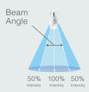
The beam angle of a light source is the angle at which the light is emitted or distributed.
